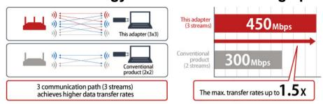
MIMO (Multiple Input Multiple Output) technology simultaneously transmits multiple data streams for increased data transfer rates. Whereas conventional 11n technology achieves speeds of 300 Mbps by transmitting dual simultaneous streams over a bandwidth of 40 MHz, this adapter simultaneously transmits three streams for transfer speeds of up to 450 Mbps, plus greater range.
