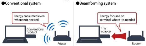
This adapter utilizes "beamforming" technology. This determines the client position and distance and focuses the signal on that location with near-pinpoint accuracy. This is effective in enhancing sensitivity and signal reception for improved wireless transmission, even in areas with numerous physical obstacles. It works especially well when paired with BUFFALO's 450 MHz router.
