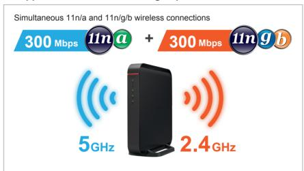
This HighPower wireless LAN router supports 802.11n/a and 802.11n/g/b 300-Mbps high-speed transfers.\* Such fast connectivity makes full use of fiber optic and other high-speed lines for easy, hassle-free downloading and data-intensive file transfers over the Internet, high- definition video playback, and more.
