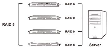
\*Combining multiple iSCSI targets requires use of operating system software RAID available in Windows 2000, XP, Vista, 7, Server 2003, and Server 2008
